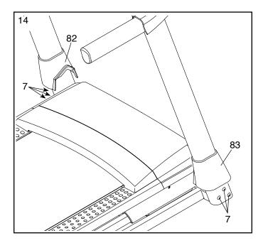
15. Make sure that all parts are properly tightened before you use the treadmill. If there are sheets of plastic on the treadmill decals, remove the plastic. To protect the floor or carpet, place a mat under the treadmill. Note: Extra hardware may be included. Keep the included hex key in a secure place; the hex key is used to adjust the walking belt (see page 24).
